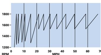
Based on 1800 RPM engine operating at 1636 RPM/62 MPH [100 kph].
